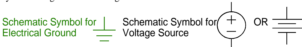
Figure 5 Schematic Symbols: GND & Voltage Source
